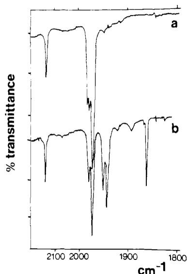
**Figure 1.** (a)  $\text{V}(\text{CO})_6$  trapped in an Ar matrix at 20 K. (b) Part a after 20-min of vacuum UV irradiation. (The band at  $\sim 2140\text{ cm}^{-1}$  is due to CO as a product of the gas-phase decomposition of the  $\text{V}(\text{CO})_6/\text{Ar}$  sample.)
