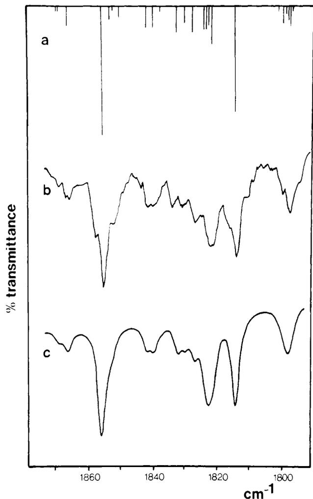
**Figure 4.** (a) Calculated "stick" spectrum (in relative optical density), (b) observed transmission spectrum, and (c) computer-simulated spectrum (Lorentzians with 3-cm<sup>-1</sup> half-width) of isotopic C<sub>4v</sub> Cr(CO)<sub>5</sub><sup>-</sup> molecules with a <sup>12</sup>CO:<sup>13</sup>CO ratio of about 1.2. Axial-equatorial angle = 95°.
