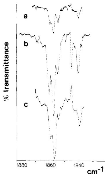
Figure 3. Infrared spectra of  $\text{Cr}(\text{CO})_5^-$  in an argon matrix produced by (a) cocondensation with sodium atoms and visible photolysis, (b) electron bombardment, and (c) vacuum-UV irradiation of  $\text{Cr}(\text{CO})_6$  in argon.
