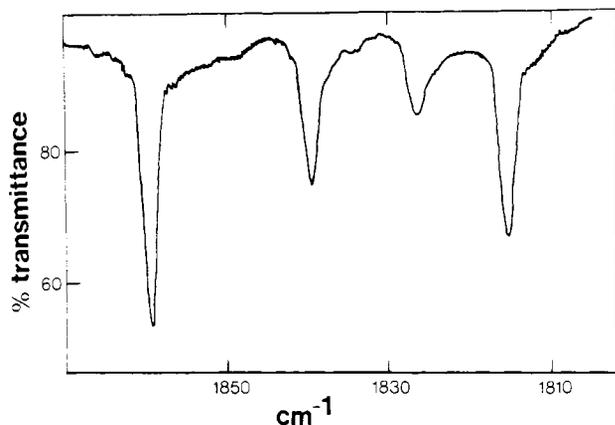
Figure 2. Isotopic spectrum of  $\text{Ni}^{(12\text{CO})_x(13\text{CO})_{3-x}-}$  molecules.
