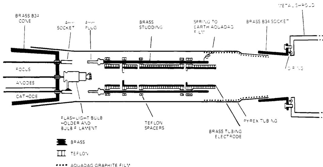
Figure 8. Electron gun assembly.
