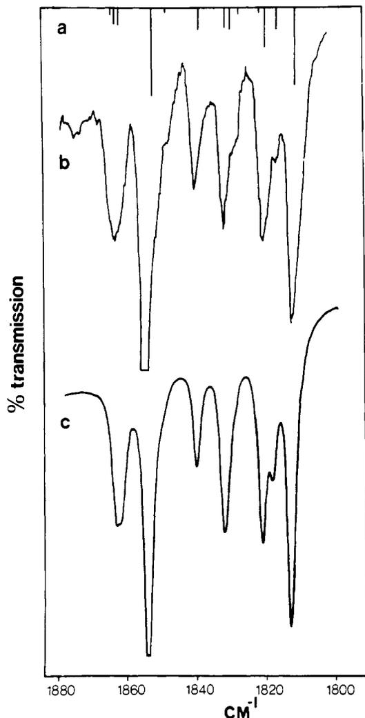
**Figure 7.** (a) Calculated "stick" spectrum (in relative optical density), (b) observed transmission spectrum, and (c) computer-simulated spectrum (Lorentzians with 3-cm<sup>-1</sup> half-width) of isotopic C<sub>3v</sub> Fe(CO)<sub>4</sub><sup>-</sup> molecules with a <sup>12</sup>CO:<sup>13</sup>CO ratio of about 1.5. Axial-equatorial angle = 103°. Compare this figure with Figure 6.
